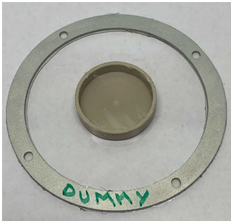
\text{Cr}_2\text{O}_3 powder pressed in a PEEK capsule & Al holder
