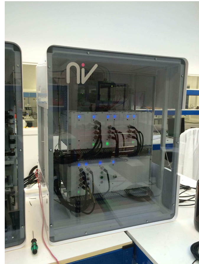
The “NiV Separator” – an innovative approach to radiochemical analysis developed by a collaboration between NNL and MicroLab Devices Ltd
